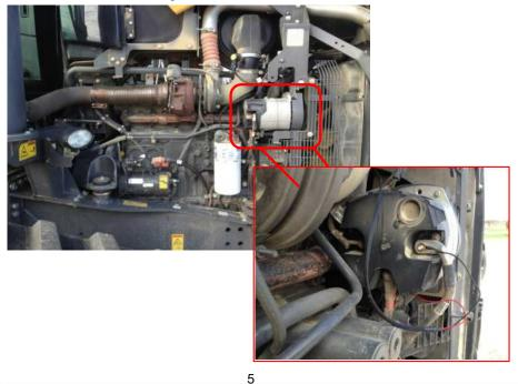
7) Plug the Harness into the module. Mount the module with supplied zip ties away from any excessive heat or moving parts. Note: Zip tie the module to the factory wire harness. Mounting the module with the connector down will help prevent moisture from collecting into the module connector.
