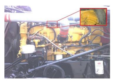
**2)** Insert the male connector of the module into the female connector on the engine. Plug the stock injector harness male connector, that was removed in Step 1, into the female connector of the module.
