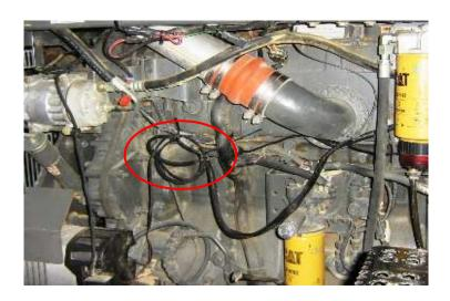
**6)** Route the power and ground wires to the alternator. Connect the red wire to +12 volts constant and the black wire to Ground.
