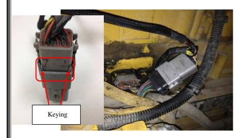
**3)** The MAP Sensor is on the same side of the engine as the air intake, and will be closer to the fan side of the engine.
