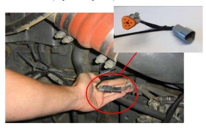
**5)** Plug the male connector on the Ag Diesel Solutions harness into the stock MAP connector. Plug the stock male MAP connector into the female connector on the Ag Diesel Solutions harness.
