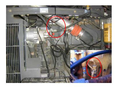
**4)** Follow the MAP Sensor wiring away from the MAP Sensor until it connects to a pigtail connector that is a 3-wire triangle-shaped connector. Unplug the triangle-shaped MAP connector.
