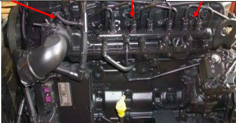
Injector connector location. Fan-side of engine.
