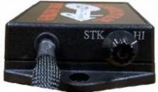
STK - Stock Mode - 0% HP Increase Position 2 - Up to 15% HP Increase HI - High Mode - Up to 30% HP Increase
