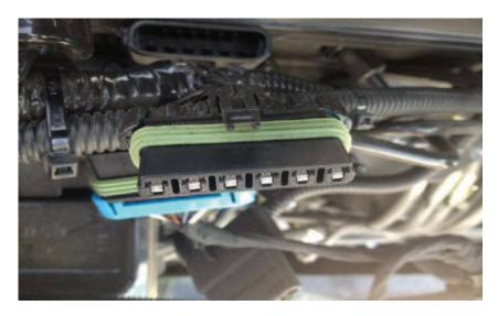
3) Plug each Male Injector Connector from the module harness into the stock location on the engine. Note: The injector connector located at the end of the module harness will plug into the injector connector located closest to the front of the engine (cooling fan side). The harness will route back toward the Cab and the module will mount near the Cab.
