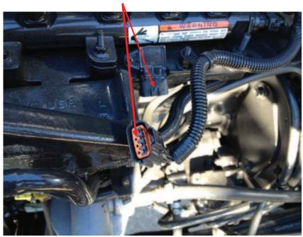
6) Connect the Male MAP Sensor plug from the module into the Stock location and the Stock Male MAP Sensor plug into the Female plug from the Module.
