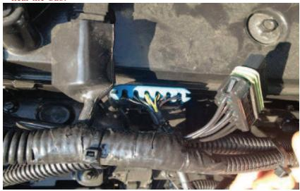
4) Connect the Stock Male Connectors, removed in Step 2, to the Female Connectors from the module harness.
