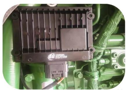
**Step 8)** Mount the module with the connector on the bottom side, as to reduce the chance of moisture from getting into the module harness. Keep away from excessive heat and moving parts.
