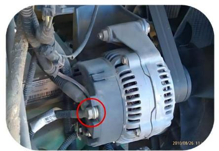
**Step 7)** Connect the red wire with the ring terminal to a +12V constant source (ie. alternator).
