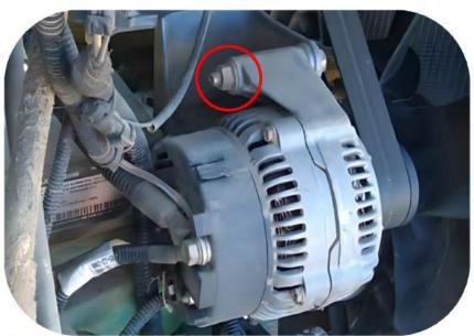
**Step 6)** Connect the black wire with the ring terminal to a good chassis ground.
