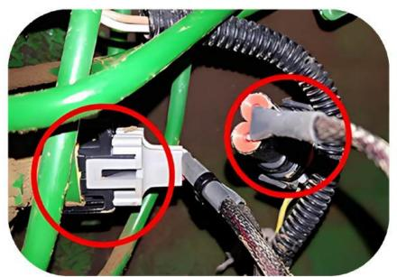
**Step 5)** Plug the male connector from the module into the DE Pump and the Male John Deere connector into the female connector from the module.
