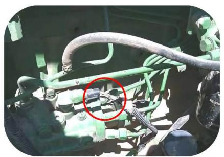
**Step 1)** From the tractor cab looking forward, locate the pump on the the left side of the engine. You will see the injector lines coming out of it.
