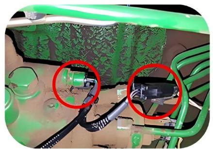
**Step 3)** Plug the male connector of the module into the pump and plug the stock John Deere connector into the female connector of the module.
