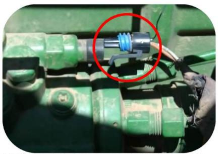
**Step 2)** Locate the fuel temp sensor at the top of the DE Pump and unplug the connector, as shown above.
