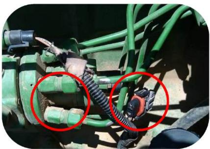
**Step 4)** Locate the fuel quantity valve connector in the center of the fuel lines and unplug the connector, as shown above.
