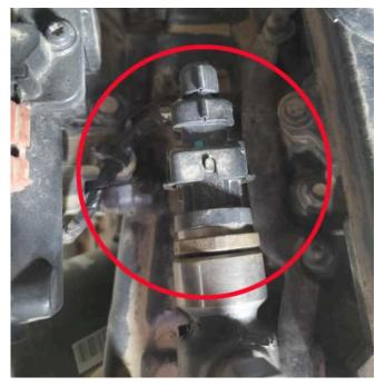
3) Unplug the stock 3-pin male connector to the fuel pressure sensor.
