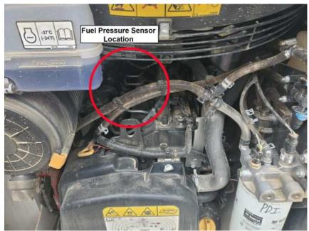
2) Locate the fuel pressure sensor as shown in the picture above. The sensor is located at the end of the common fuel rail.
