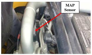
**6)** Remove the factory four- pin male connector located on the engine harness from the MAP sensor. Press and release the locking tab to disconnect.
