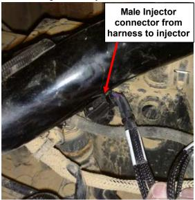
**4)** Connect the male two pin connectors from the factory harness to the female injector connectors on the ADS harness. **Note:** Insure that all connectors snap and fasten securely.
