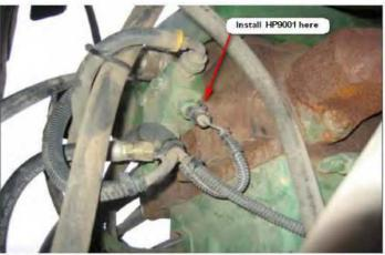
Mount module in a secure location. Zip tie module and any loose wires down.
