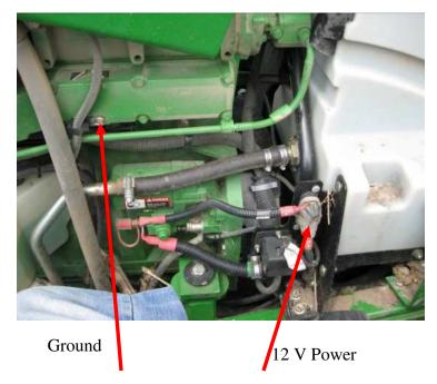
8) Connect the black wire with ring terminal to a good chassis ground
