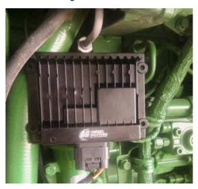
**10)** Mount the module with the connector on the bottom side, as to reduce the chance of moisture from getting into the module harness. Keep away from excessive heat and moving parts.
