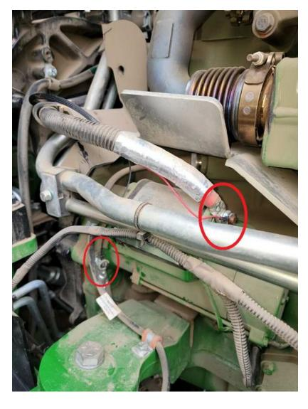
**9)** Connect the harness into the module. Mount the module and harness away from any excessive heat or moving parts. Note: Mounting the module with the harness connector down will help prevent moisture from collecting into the module connector.
