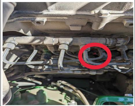
4) Pull back dust boot, red locking tab and disconnect connector.
