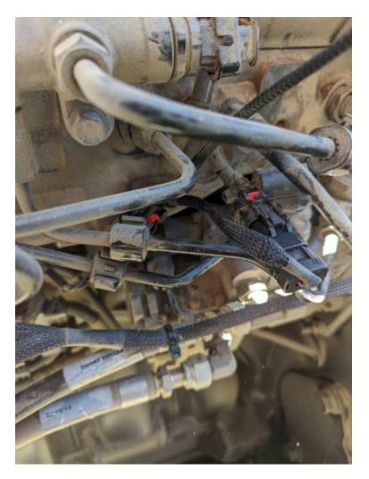
NOTE: BE SURE TO FULLY ENGAGE CONNECTORS AND RED LOCKING TABS. 6) Route power and ground leads over to the starter.
