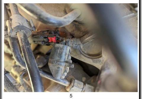
**5)** Connect the module male connector into fuel pressure sensor female pigtail. Connect the module female connector into fuel pressure sensor factory wiring harness male connector.
