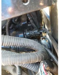
**5)** Connect the stock female connector to the male fuel pressure connector from the module harness. Make sure the connectors go together smoothly and you hear an audible 'click'.
