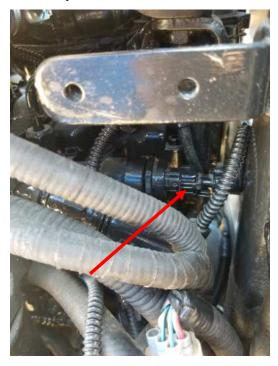
**4)** Plug female fuel pressure connector from module into fuel pressure sensor. Make sure the connector plugs in smoothly and you hear an audible 'click'.
