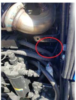
3) Press down on tab to unplug fuel pressure sensor. If the plug seems stuck pushing the connector into the rail while holding the release tab can sometimes help it unlatch.
