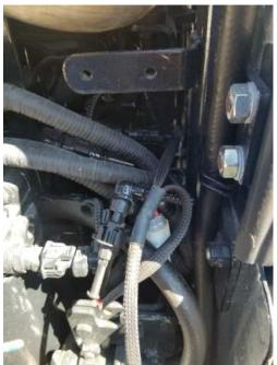
**6)** Mount module in a secure location away from any extreme heat or moving parts. Secure the module and any excess harness with supplied zip ties.
