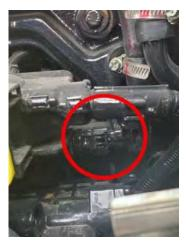
**3)** Connect the 3-Pin male fuel pressure connector on the Ag Diesel Solutions Module to the stock 3-Pin female connector on the engine. Then connect the stock 3-Pin male connector on the engine harness to the 3-pin female connector on the Ag Diesel Solutions module Harness.
