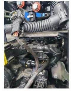
**4)** Mount the module with the connector on the bottom side, as to reduce the chance of moisture from getting into the module harness. Keep away from excessive heat and moving parts. Note: Zip tie onto the factory computer wire harness works well. Mounting the module as shown will help prevent moisture from collecting into the module connector.
