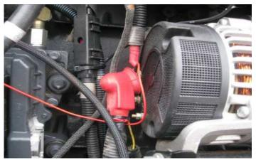
9) Plug the harness into the module. Mount the module with supplied zip ties away from any excessive heat or moving parts. Note: Zip tie the module to the factory wire harness. Mounting the module with the switch connector down will help prevent moisture from collecting into the module connector.
