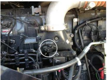
**6)** Plug the male MAP sensor from the Ag Diesel Solutions module into the stock location and the stock male MAP sensor into the female connector.
