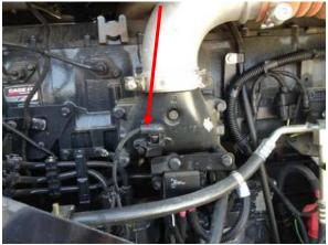
**6)** Plug the male MAP sensor connector from the module into the stock location and the stock male MAP sensor connector into the female connector from the module.
