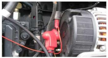
**9)** Mount the module with the connector on the bottom side, as to reduce the chance of moisture from getting into the module harness. Keep away from excessive heat and moving parts. Note: Zip tie onto the factory computer wire harness works well. Mounting the module as shown will help prevent moisture from collecting into the module connector.
