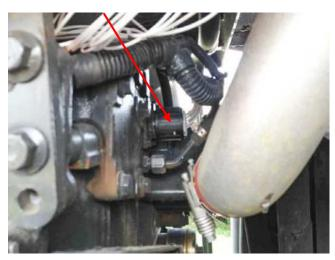
**3)** Plug the male connector from the Ag Diesel Solutions module into the stock location on the engine head. Align the inside section of the connector to the stock plug and then rotate the outer shell clockwise to tighten.
