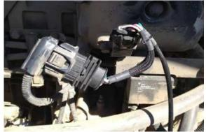
7) Connect the Black wire with Ring Terminal to a good Chassis ground8) Connect Red wire with ring terminal to a 12V constant source (i.e. alternator)
