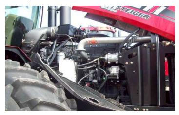
**2)** Unplug the stock injector connector from the front side of the engine head. To loosen, rotate the outer shell of the connector counter-clockwise.
