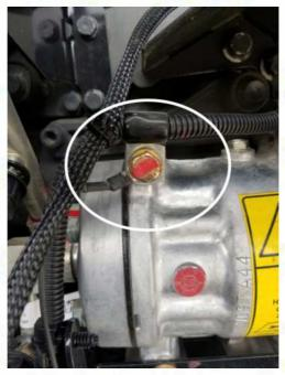
**9)** Plug the harness into the module. Mount the module with supplied zip ties away from any excessive heat or moving parts. Note: Zip tie the module to the factory wire harness. Mounting the module with the switch connector down will help prevent moisture from collecting into the module connector.
