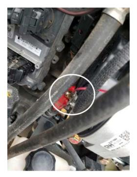
**8)** Connect the Black wire with Ring Terminal to a good chassis ground. Note: Make sure ground surface is clean metal to metal contact. Even if surface underneath painted components seems clean, abrasive cleaning or alternate location is recommended.
