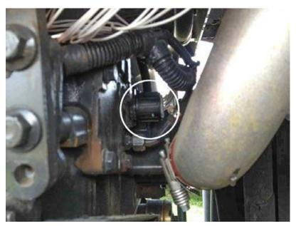
**3)** Plug the female connector from the Ag Diesel Solutions harness into the stock location on the engine head. Align the inside section of the connector to the stock plug and then rotate the outer shell clockwise to tighten. Note: The outer shell spins free of the inside connector. Align the inside section and rotate the outer shell until the connector locks in place.
