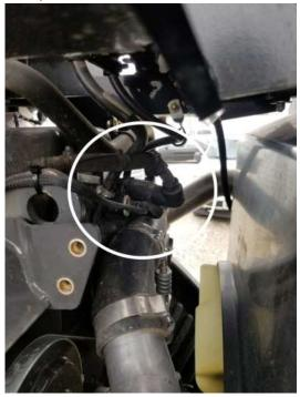
**5)** Unplug the stock female MAP sensor by depressing the release tab and pulling back on connector.
