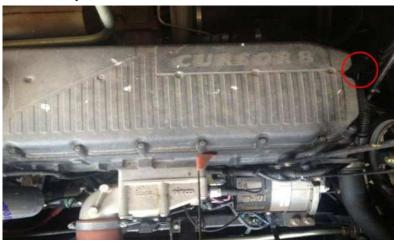
**2)** Unplug the round millitary style injector connector. Channel locks or large pliers may be needed to loosen the connector.
