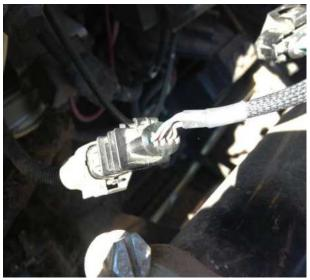
**6)** Plug the male MAP sensor connector from the module harness into the stock MAP sensor.
