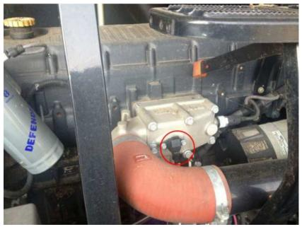
**5)** Plug the female MAP sensor connector from the module harness into the stock MAP sensor connector.
