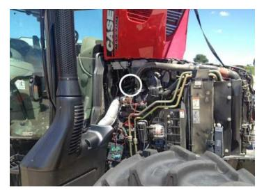
**2)** The ECM is mounted on a bracket that sits above the engine. Locate the MAP sensor, and power and ground as shown in picture below.
