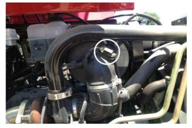
**7)** Unplug the MAP sensor and plug male connector from the Ag Diesel Solutions module into the MAP sensor. Plug the female connector from the Ag Diesel Solutions module into the stock MAP sensor wiring harness.
