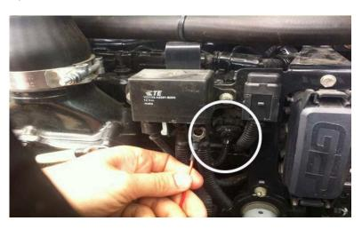
**8)**Plug the Ag Diesel Solutions female MAP sensor into the stock male MAP Sensor. Plug the new male MAP sensor into the stock female MAP sensor.
