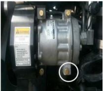
**10)** Plug the Harness into the module. Mount the module with supplied zip ties away from any excessive heat or moving parts. Note: Zip tie the module to the factory wire harness. Mounting the module with the connector down will help prevent moisture from collecting into the module connector.
