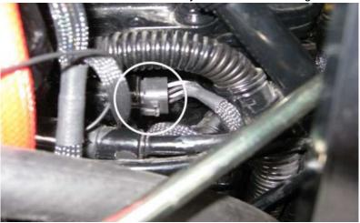
**6)** Continue to the next set of injector connectors. Repeat Steps 4 and 5 to connect the injector connectors.
