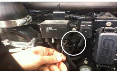
**8)** Plug the Ag Diesel Solutions female MAP sensor into the stock male MAP Sensor. Plug the new male MAP sensor into the stock female MAP sensor.
