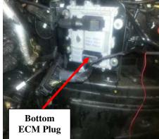
**3)** Plug the male connector from the Ag Diesel Solutions module into the ECM.
