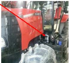
2) Unplug the stock ECM harness by rotating the locking lever to release. The correct connector is located on the bottom of the ECM. Remove the harness from the ECM. Note: if the ECM is mounted on the side of the engine, the correct connector is located at the top of the ECM. If the ECM is located in a sealed box by the cab, the correct plug is located at the bottom of the ECM.
