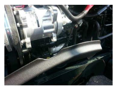
7) Mount the module with the connector on the bottom side, as to reduce the chance of moisture from getting into the module harness. Keep away from excessive heat and moving parts. Note: Zip tie onto the factory computer wire harness works well. Mounting the module as shown will help prevent moisture from collecting into the module connector
