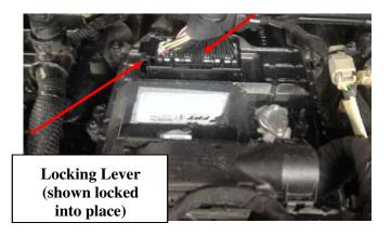
**4)** Plug the stock male connector located on the engine harness into the female connector on the module harness. Gently push the connectors together while you rotate the locking lever to latch the connectors together.
