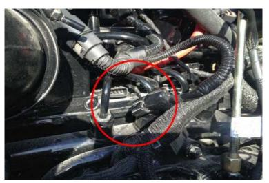
**8)** Plug the male MAP sensor into the stock MAP Sensor. Connect the female MAP sensor into the stock MAP sensor wiring.
