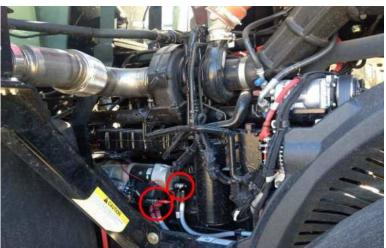
**10)** Plug the harness into the module. Mount the module, with supplied zip ties, away from any excessive heat or moving parts. Note: Zip tie the module to the factory wire harness. Mounting the module with the switch connector down will help prevent moisture from collecting into the module connector.
