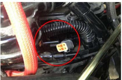
**3)** Route the harness as shown in the picture below. The module Case will be located closer to the Flywheel side of the engine.
