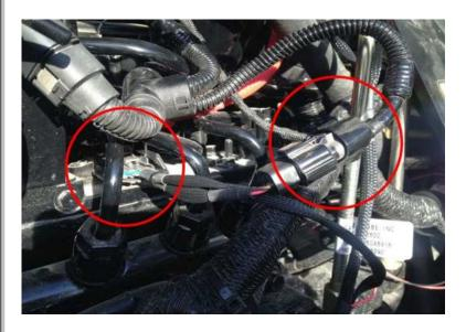
**9)** Connect the Red wire with ring terminal to a +12V constant source. Connect the Black wire with ring terminal to a good Chassis Ground. (The Starter is the best possible connection).
