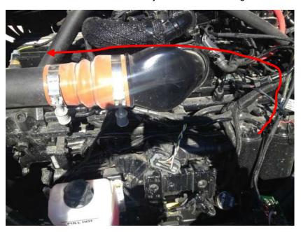
**4)** On the Ag Diesel Solutions harness, the female injector connector located closest to the module will connect to the male injector connector wiring located closest to the Flywheel-side of the engine.
