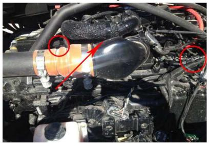
**2)** Unplug all 3 sets of injector connectors. Press the release tab on the connector and gently pull the connector apart.
