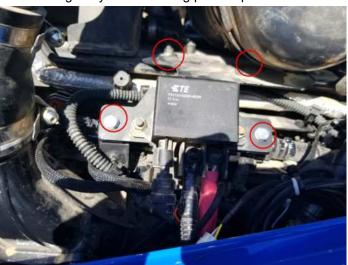
**3)** On the Ag Diesel Solutions harness, the male injector connector located farthest from the module will connect to the female injector connector located closest to the fan side of the engine. Plug the stock male injector connector into the Ag Diesel Solutions female injector connector. Repeat this for the other 2 set of injector connectors.
