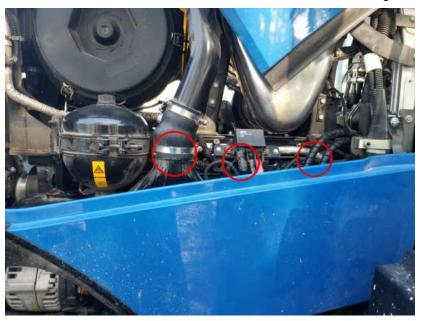
**2)** To better access the injector connectors, remove 2 bolts and nuts holding relay and mounting plate in place.
