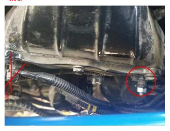
**6)** Install red 12V module power wire to alternator or other constant 12V source.
