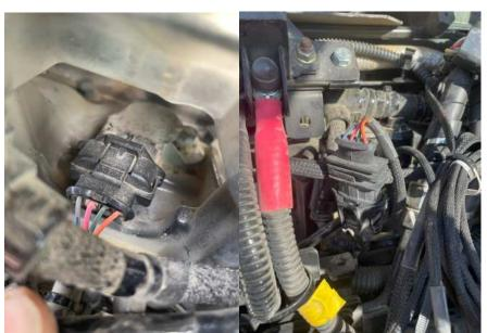
**5)** Remove ground strap on right side (circled below) of intake horn. Use sandpaper or other abrasive to remove paint from surface and install black module ground wire.
