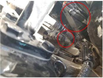
**4)** Plug the module male MAP sensor connector into the stock female MAP sensor. Plug the stock male connector into the module female connector.
