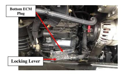
**3)** Plug the male connector from the Ag Diesel Solutions module into the ECM.
