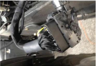
**5)** Route the red power wire to the alternator, +12 volt constant source. The black wire will connect to a good ground.
