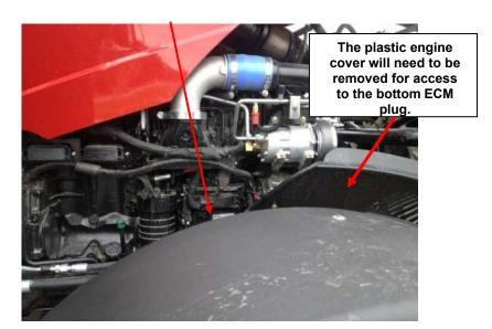
**2)** Unplug the stock ECM harness by rotating the locking lever to release. The correct connector is located on the bottom of the ECM. Remove the harness from the ECM.
