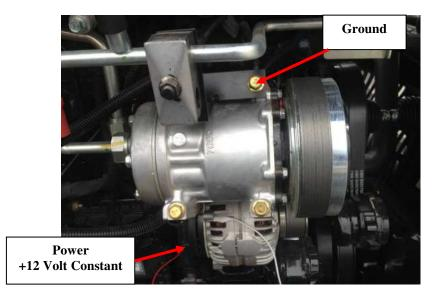
**6)** Mount the module with the connector on the bottom side, as to reduce the chance of moisture from getting into the module harness. Keep away from excessive heat and moving parts. Note: Zip tie onto the factory computer wire harness works well. Mounting the module as shown will help prevent moisture from collecting into the module connector
