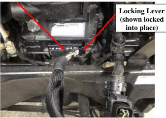
**4)** Plug the stock male connector located on the engine harness into the female connector on the module harness. Gently push the connectors together while you rotate the locking lever to latch the connectors together.
