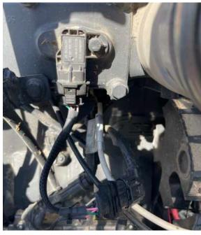
**6)** Connect the Black and Red wire with Ring Terminals to an engine ground and constant 12 Volt Source (ie. Alternator)
