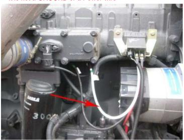
7) Plug the harness into the module. Mount the module with supplied zip ties away from any excessive heat or moving parts. Note: Zip tie the module to the factory wire harness. Mounting the module with the switch connector down will help prevent moisture from collecting into the module connector.
