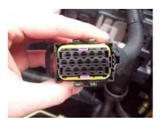
3) Plug the stock connector into the Ag Diesel Solutions female connector. Plug the Ag Diesel Solutions male connector into the ECM. **Note:** Make sure to push completely together until the connector snaps.
