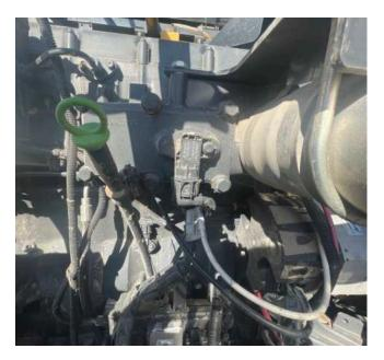
5) Plug the stock male MAP connector into the female connector
