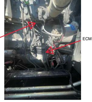
**2)** Unplug the small connector on on the top left of the ECM with 16 pins in it, you will need to unplug the bottom first. Ensure Purple Tabs are in center location.
