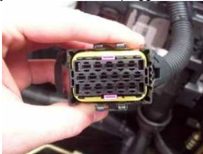
Factory Iveco connector unplugged from ECM
