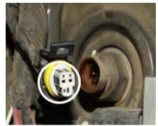
**7)** Plug in the Ag Diesel Solutions male connector into the stock MAP sensor
