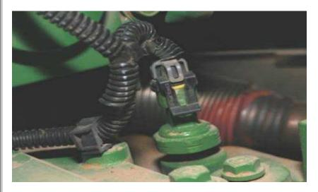
**8)** Plug the stock MAP sensor connector into the Ag Diesel Solutions female map sensor connector.
