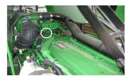
**6)** Check inside the MAP Sensor for a plastic insert. If there is a plastic insert, you will need to remove it and place it over the stock MAP Sensor.
