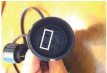
Note: Rotate the collar on the factory John Deere connector clockwise 2 or 3 degrees as shown in picture below before connecting to the male connector on the module
