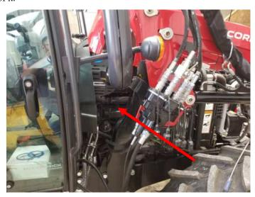
2) Locate fuel pressure sensor as shown below. It can be found at the end of the fuel rail closest to the cab.
