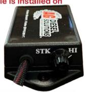
STK- Stock Mode - 0% HP Increase Position 2- Up to 15% HP Increase Hi - High Mode - up to 30% HP Increase
