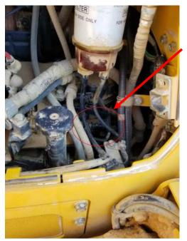
3) Press down on tab and pull to unplug the fuel pressure sensor connector.
