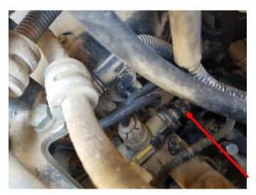
**4)** Plug Female Fuel Pressure Connector from module into fuel pressure sensor.
