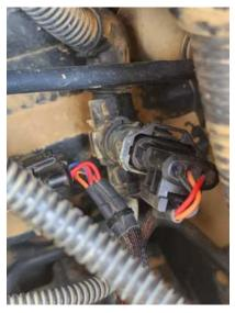
**6**) Mount module in a secure location. Zip tie module and any loose wires down away from heat and moving parts.
