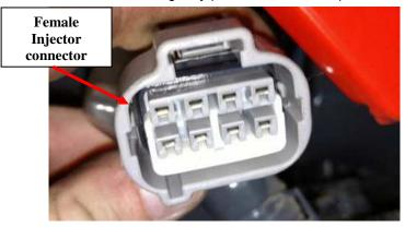
3) On the Ag Diesel Solutions module harness, the grey 8 pin male injector connector will connect to the female injector connector fixed on the engine. The Ag Diesel Solutions module harness can be routed along existing wire loom.
