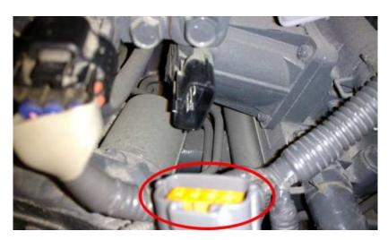
**7)** Plug the new male EGR Valve connector from the module harness into the stock female EGR Valve. Plug the Ag Diesel Solutions female EGR Valve connector from the harness into the stock male EGR Valve connector.
