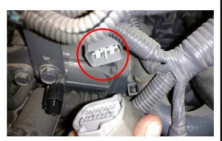
**4)** On the module harness, the 8 pin female Injector connector will now connect to the factory male Injector connector that was unplugged from the engine in step 3.
