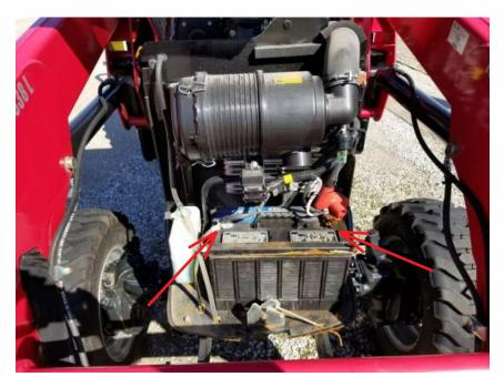
4) Run the power and ground leads directly to the battery.
