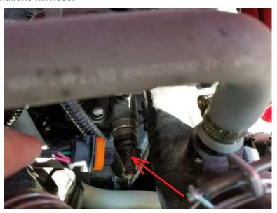
**3)** Locate and unplug the 3 injector connectors. Plug the Ag Diesel Solutions male connectors into the stock female injectors. Then plug the stock male connectors into the Ag Diesel Solutions harness.
