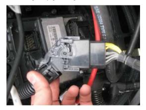
5) Unplug MAP sensor and Plug Female connector from module into the Map Sensor, then connect the Female Map Connector to the Male connector of the module.
