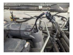
6) Connect the Black wire with Ring Terminal to a good Chassis ground
