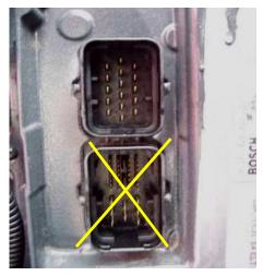
3) Plug the Female connector from the module into the 16 pin ECM port.
