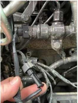
**5)** Mount module in a secure location away from any extreme heat or moving parts. Zip tie module and any loose wires down.
