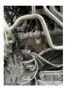
2) Locate the fuel pressure sensor as shown in the picture above. The sensor is located at the end of the common fuel rail.
