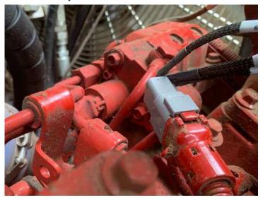
**6)** Locate the MAP sensor. The MAP sensor is located between the fuel rail and the injector connector on the Flywheel side of the engine.
