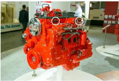
**3)** Unplug both sets of stock injector connectors. Press the release tabs on the connector and gently pull the connectors apart.
