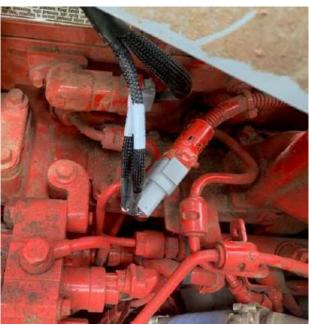
**5)** Plug both of the Ag Diesel Solutions female injector connectors into the factory wire harness.
