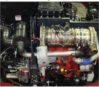
**2)** Locate the 2 stock injector connectors attached to the side of the engine head. These are located on the side with the air intake opposite the turbocharger. One connector is located closer to the Flywheel side of the engine and the other connector is located closer to the Fan side of the engine.
