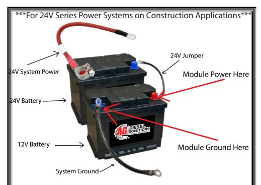
Module power and ground must be hooked to the 12V side of a 24V series power system for the module to function properly. Module ground lead needs to be hooked to the system ground which will be the battery with its ground strap connected to the frame of the machine NO the jumper running between batteries. The module power lead needs to be hooked up to the positive terminal WITH the jumper (on same battery), NOT the 24V System power terminal. Please see illustration above.
