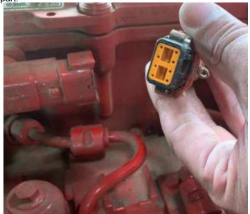
**4)** Plug both of the Ag Diesel Solutions male injector connectors into the fan and flywheel connectors coming out of the engine head.
