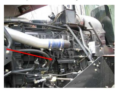
2) Locate Fuel Quantity Valve sensor as shown in Picture
