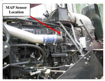
**6**) Locate MAP sensor on left side of engine in the air intake manifold
