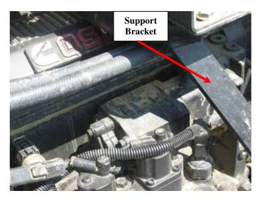
Mount the module box in a safe location using the zip ties to secure the wires and module away from any extreme heat and moving parts. A good location to mount the module is on the given support bracket.
