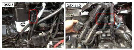
**5)** Route the power and ground wires to the starter located on the driver's side between the frame rail and engine.
