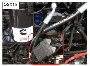
Note: For the QSX11.9, both ECM connectors will need to be removed for proper installation of the harness to the ECM.
