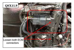
**4)** Plug the Ag Diesel Solutions male harness into the stock female connector located on the ECM Engine Connector 1. Refer to the diagram in Step 2 for correct location of ECM connector.
