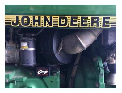
6) Mount the module case in a safe location using the supplied zip ties to secure the wires and module away from any extreme heat and moving parts.
