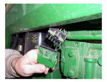
**3)** Disconnect the factory Male and Female fuel pump connectors.
