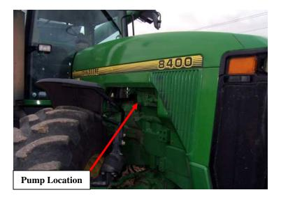
Locate Bosch P-pump on left side of tractor beside the front tire, if you're facing the front of the tractor.
