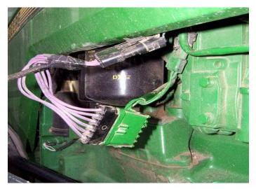
5) Insert the Male connector from the ADS module harness into the factory Female fuel pump connector.NOTE: Make sure to push completely together until the connector snaps.
