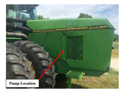
1) Locate Bosch P-pump on left side of tractor behind the hood door, if you're facing the front of the tractor.
