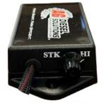
STK- Stock Mode - 0% HP Increase Position 2- Up to 15% HP Increase Position 3- Up to 25% HP Increase HI - High Mode - up to 35% HP Increase
