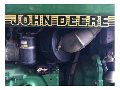
6) Mount the module case in a safe location using the supplied zip ties to secure the wires and module away from any extreme heat and moving parts.
