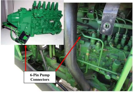
2) Locate the 6-Pin fuel pump connector coming off of the back of the fuel pump as shown in the picture above.
