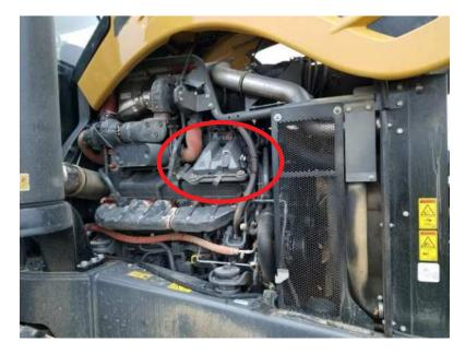
You will be working on both sides of the tractor as it works off of two ECM controllers. Picture above is the "passenger" side and the ECM is in plan view. You will have to remove the plastic cover to access the ECM harness plug.
