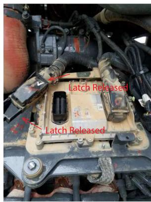
After you have released the factor ECM Plug, you can install our ECM plug in its place and slide the latch back in to fully seat the new connector to the ECM. Take your time and get everything lined up and it will pull itself together, do not force the connectors together.
