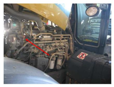
**9)** Mount the module with the connector on the bottom side, as to reduce the chance of moisture from getting into the module harness. Keep away from excessive heat and moving parts. Note: Zip tie onto the factory computer wire harness works well. Mounting the module as shown will help prevent moisture from collecting into the module connector.
