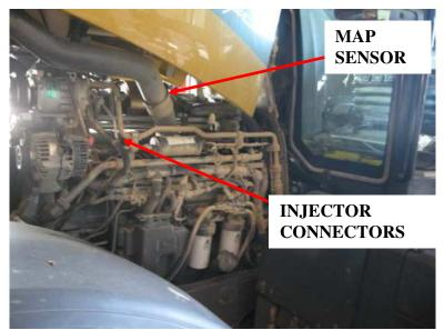
**3)** Plug MAP sensor connector from module into MAP sensor and plug the MAP harness from engine into Module
