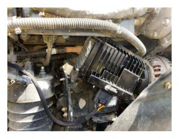
**Step 9)** 9) Mount the Ag Diesel Solutions module with the provided zip ties in a secure and dry location.
