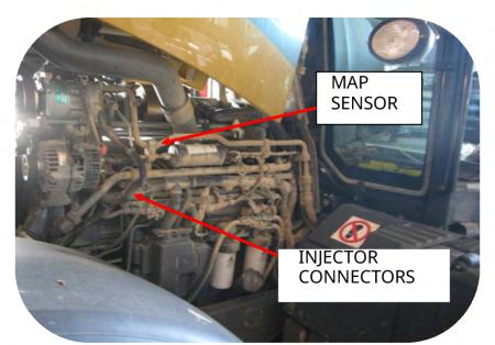
**Step 1)** From the tractor cab looking forward, locate the fuel system on the left side of the engine. You will see the common rail with the injector lines coming out of it.
