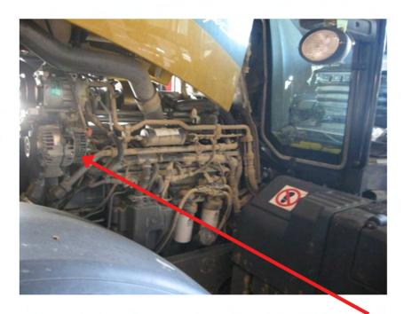
**Step 7)** Connect the black wire with ring terminal to a good chassis ground.
