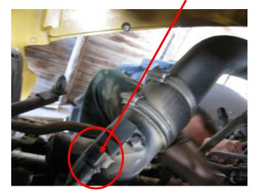
3) Plug MAP sensor connector from the Ag Diesel Solutions module into MAP sensor. Plug the MAP connector from engine harness into the module.
