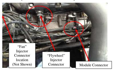
4) On the new harness, the female Injector Connector located closest to the Module will plug into the "Flywheel" Injector Connector on the engine head. The female Injector Connector located furthest from the Module will plug into the "Fan" Connector on the engine head. The Male connectors plug into the Stock Injector connectors removed in Step 2.
