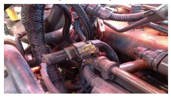
8) Connect the Red wire with ring terminal to a +12V constant source. Connect the Black wire with ring terminal to a good Chassis Ground. (The Alternator is the best possible connection).
