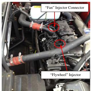
2) Disconnect both Fan and Flywheel connectors. Rotate the outer collar of the injector connectors counter-clockwise to loosen from the side of the engine
