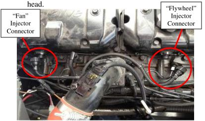
3) Facing the side of the engine, route the Module Harness as shown in the pictures below. The Module Connector will be located to the Right of the Injector Connector labeled "Flywheel".
