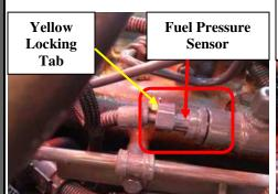
Fuel Pressure connector from module connected to stock Fuel Pressure Sensor.
