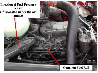
6) Disconnect the stock Fuel Pressure Sensor connector, move the Locking Tab to release. Plug the male connector from the module harness into the Stock Fuel Pressure Sensor.
