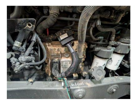
Step 3) Disconnect Left ECM connector by rotating the locking lever up to release factory connector.
