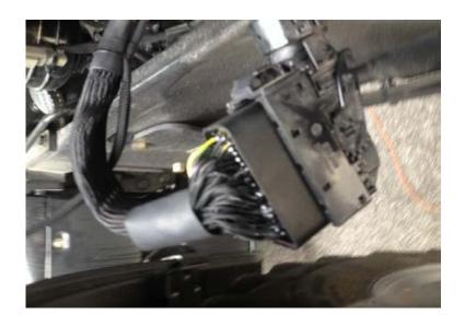
Step 5) Plug the stock female connector located on the engine harness into the male connector on the module harness. Gently push the connectors together while you rotate the locking lever to latch the connectors together.
