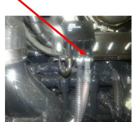
Step 8) Connect the black ground wire to a good clean ground. the air conditioner compressor mounting bolt can be used.
