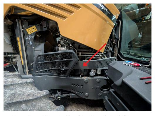
**Step 1)** Locate ECM on the driver side of the engine behind these panels.
