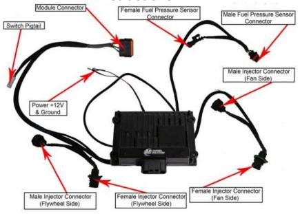
1) Locate the 2 sets of injector connectors on the side of the engine head.
