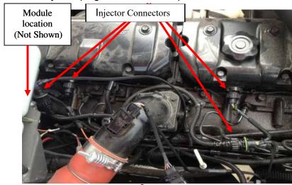
**5)** Locate the fuel pressure sensor. It is located at the end of the common fuel rail.
