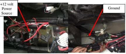
**9)** Plug the harness into the module. Mount the module with supplied zip ties away from any excessive heat or moving parts. Note: Zip tie the module to the factory wire harness. Mounting the module with the connector down will help prevent moisture
