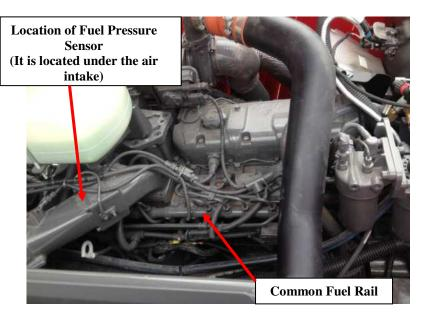
**6)** Disconnect the stock fuel pressure sensor connector, squeeze the locking tab to release. Plug the male connector from the module harness into the stock fuel pressure sensor.
