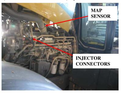
**3)** Plug MAP sensor connector from module into MAP sensor and plug the MAP harness from engine into Module
