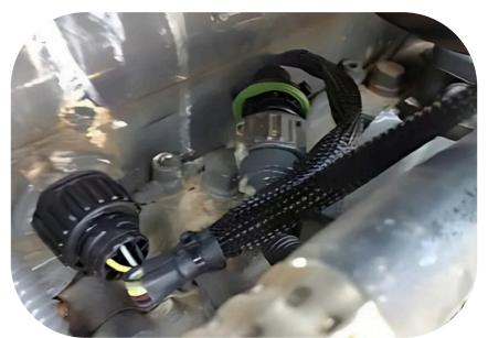
**Step 5)** Insert the male injector connector from the Ag Diesel Solutions Module harness into the female injector connector on the cylinder head. Insert the female connector from the Ag Diesel Solutions module harness into the male injector connector on the engine harness.
