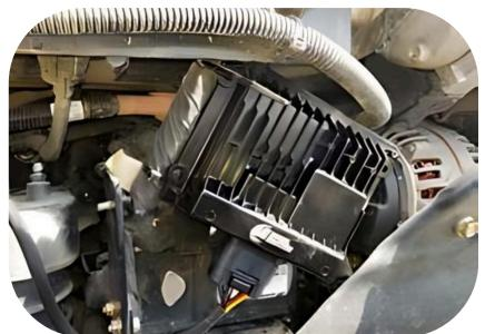
Step 7) Mount the module with the connector on the bottom side, as to reduce the chance of moisture from getting into the module harness. Keep away from excessive heat and moving parts.
