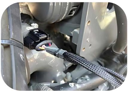
**Step 2)** Locate the factory MAP Sensor connector on the intake manifold and unplug.
