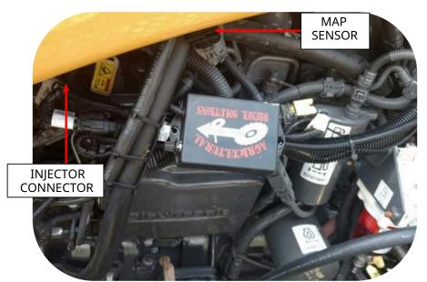
**Step 1)** From the cab looking forward, locate the fuel system on the left side of the engine. You will see the common rail with the injector lines coming out of it.
