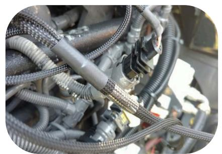
**Step 3)** Insert the male MAP sensor connector from Ag Diesel Solutions module into the MAP sensor on the intake. Connect the factory male MAP sensor connector from the engine into the female connector on the Ag Diesel Solutions module harness.
