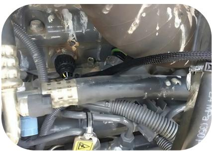
**Step 4)** Locate the factory Injector Connector on the side of the cylinder head.
