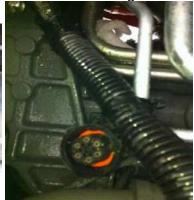
6) Route the power and ground straps across the engine to the alternator. Connect the **Black** wire with ring terminal to the mounting bolt on the alternator. Following, connect the **Red** wire with ring terminal to a 12V constant source on the alternator (+ terminal.)
