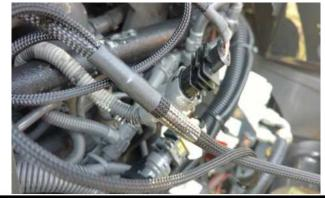
**4)** Locate the factory Injector Connector on the side of the cylinder head.
