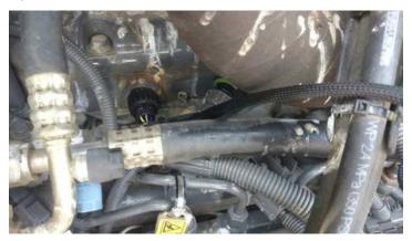
**5)** Insert the male injector connector from the Ag Diesel Solutions Module harness into the female injector connector on the cylinder head. Insert the female connector from the Ag Diesel Solutions module harness into the male injector connector on the engine harness.
