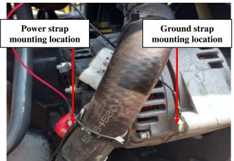
7) Mount the module with the connector on the bottom side, as to reduce the chance of moisture from getting into the module harness. Keep away from excessive heat and moving parts.
