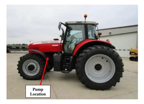
1) From the tractor cab looking forward, locate the pump on the left side of the engine. You will see the injector lines coming out of it.
