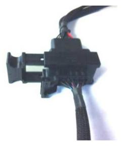
4) Connect the stock female pump connector to the male pump connector on the Ag Diesel Solutions module harness.
