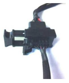
4) Connect the stock Female pump connector to the Male pump connector on the ADS module harness.
